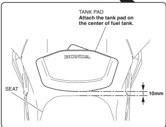
4. Apply adequate pressure to the attached tank pad.
