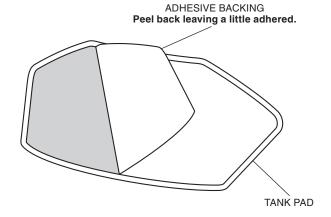
3. Attach the tank pad and remove the adhesive backing as shown.
