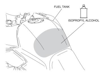
2. Peel off the adhesive backing on the tank pad as shown.
